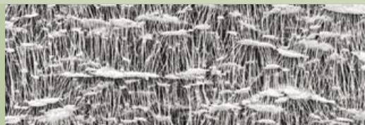
Tetratex PTFE membrane 250x magnification
